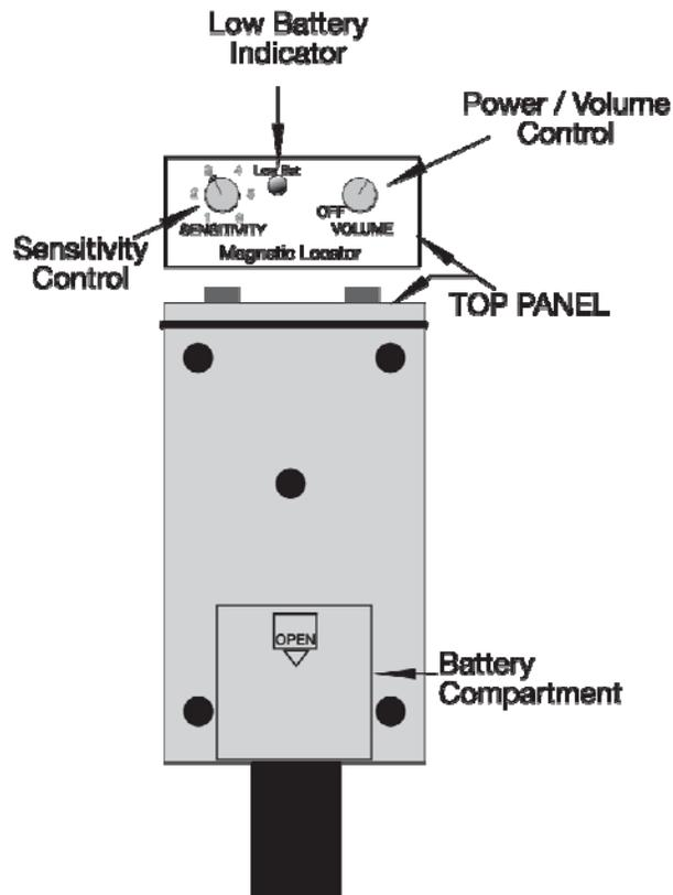
Figure 2: Instrument Controls
